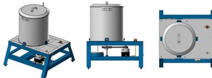
Gambar 3. Desain mesin spinner pulling oil tampak:(a)isometrik, (b)samping dan (c)atas
