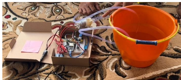
Gambar 3. Ujicoba prototipe Smart Plant Monitoring berbasis ESP32
